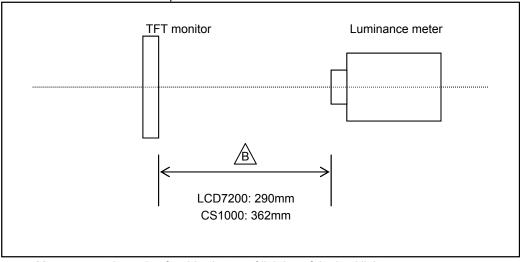
Measurement is made after 30 minutes of lighting of the backlight.
